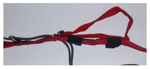
Place the excessive line in the pocket on the rear side of the riser.
