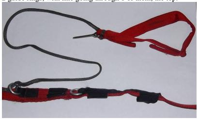
For stowing, fold the line in the stow loop point in half, insert into bottom ring.
