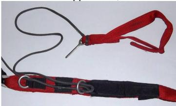
Put the pin into the stow loop, under the ring, than above it.
