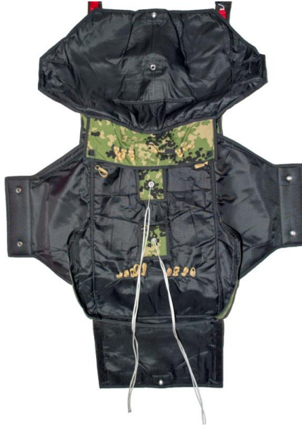
Picture 17. Straightening the Canopy
