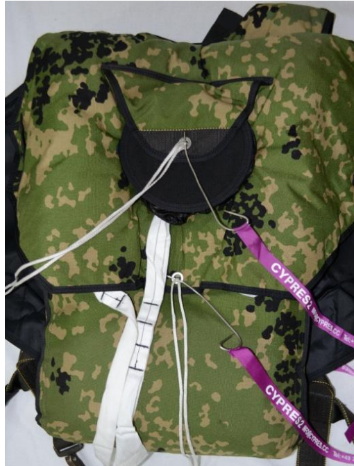
Picture 27. Closing the Upper PC Protector Flap
