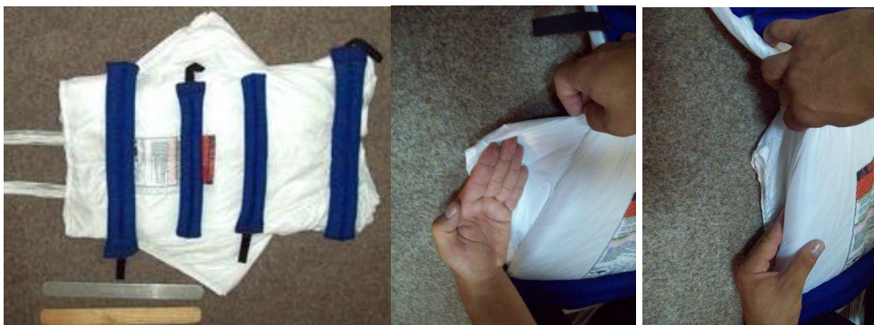
Picture 12 d. Flaking the Canopy
